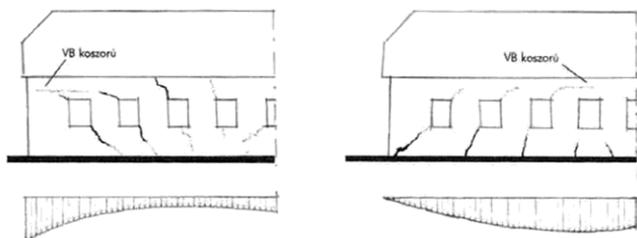
Figure 3. Rate of sinking depending on cracks [6]
