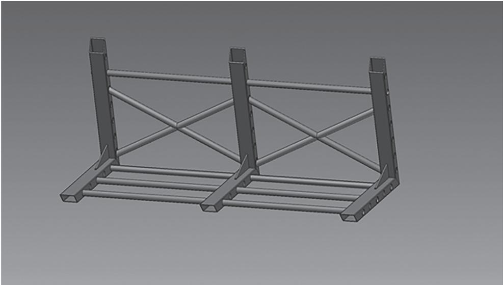
Figure 1. *Anti VBIED Obstacle developed by the University of Defence.*
