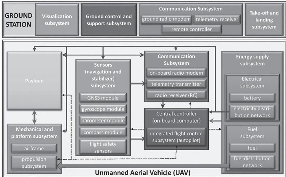
Figure 3. A generalized UAS structure.
